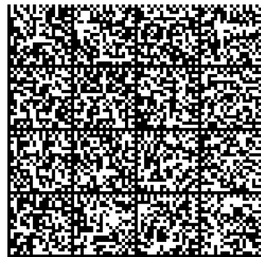
A Data Matrix containing 560 characters, readable when scanned at 200 dpi.
