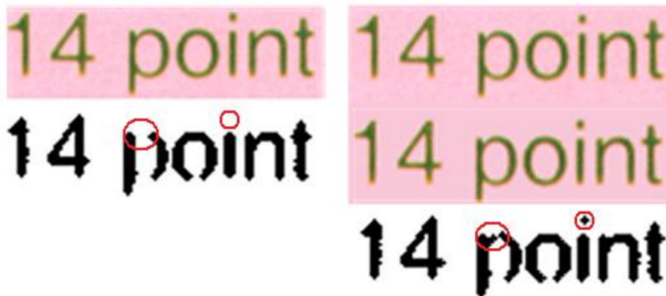
Figure 3 Binarizing alone (left) compared to Image Detergent followed by binarization (right). The thin areas of the characters proved difficult for the binarization process, but a cleaned image resulted in fewer broken characters.
