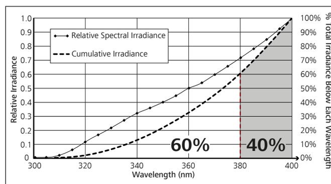
Figure 2. ISO 8980-3 solar UVR spectrum normalized to its maximum value at wavelength of 400 nm.
