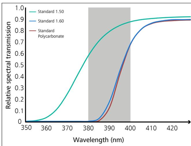
Figure 11a. Standard lens materials pass significant amounts of UVR.
