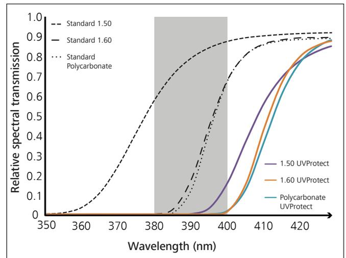
Figure 11b. ZEISS UV Protect materials pass only visible light.
