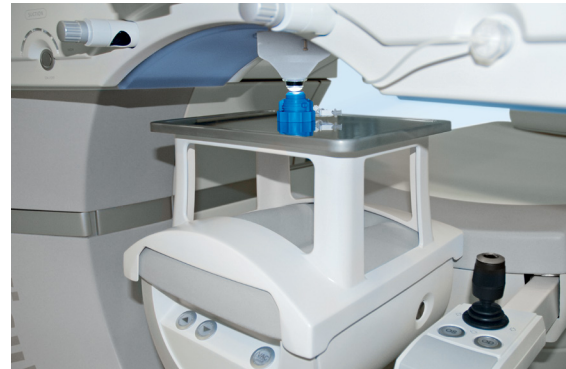
The unique adapter attached to the headrest of the patient supporting system serves as an ideal work platform for preparing the corneal donor graft
