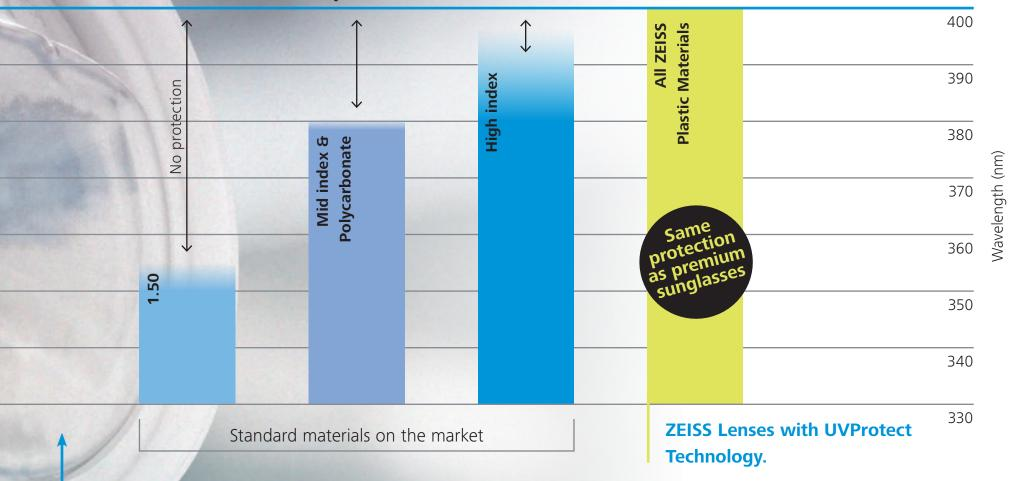
**Protection is cast into the lens material when being molded.**  UV
