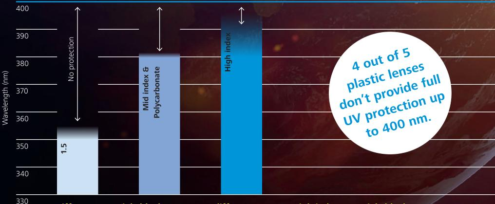
Different materials block UV rays to different extents. High index materials block UV almost completely, whereas low index materials do not.
