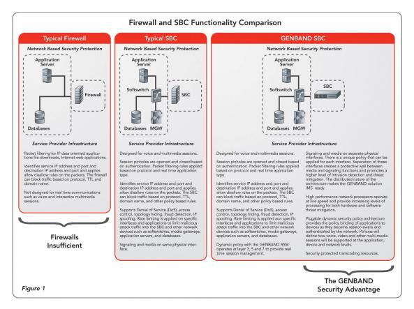
The SBC is positioned at the IP network border and peering point to protect many types of service provider networks. The SBC provides the security function for both fixed and mobile networks including residential and business, federated exchanges, directory and contact centers.
