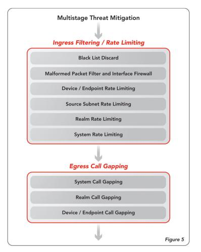
The second and subsequent layers at ingress are for rate limiting at a system/interface, realm and device level for "known" devices. This allows for rate policies to be applied at any desired granularity.
