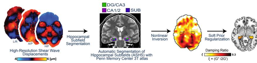
**OUTCOME MEASURE:** Damping ratio; lower damping ratio measures are indicative of better structural integrity
