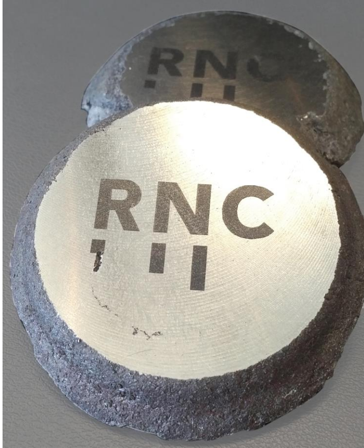
Ferro-nickel puck produced from Dumont concentrate
