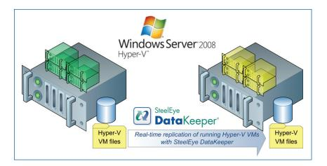
volume resource. Any application that can be clustered with WSFC can now be further protected by replacing the single point of failure of the shared Physical Disk resource with a DataKeeper volume resource. Regardless of whether it is Exchange, SQL, IIS, File Print, Hyper-V or any other WSFC protected application, DataKeeper works seamlessly with WSFC to enhance the availability of that application.
