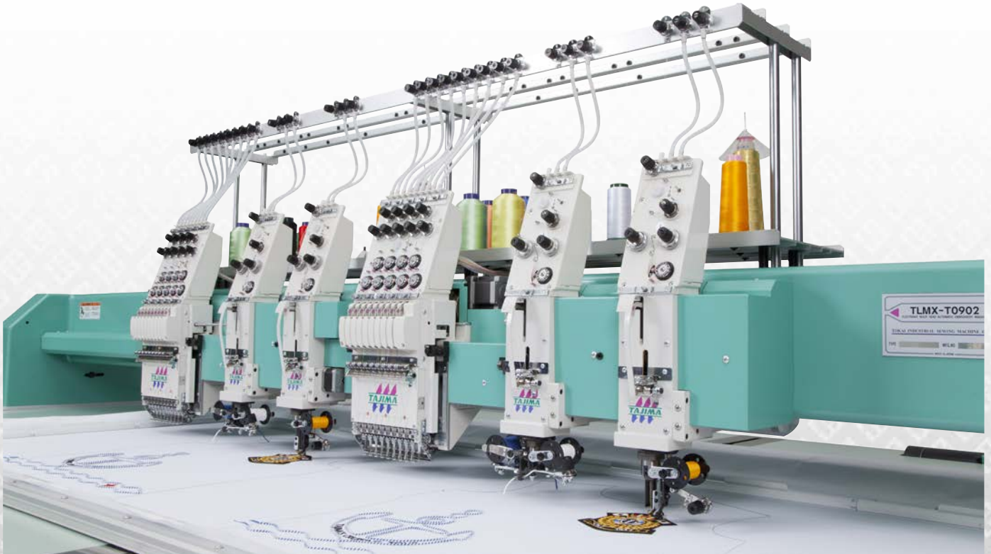
TLMX TRIPLE MIXED TYPE MACHINE: 2 LOCK STITCH CHENILLE + 1 MULTI COLOR HEAD
