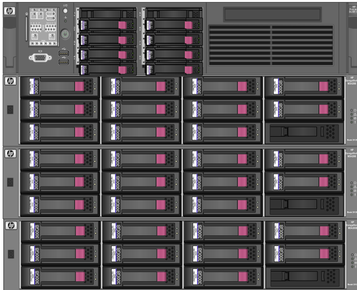
Figure 1. Fast Track 6TB reference architecture with the ProLiant DL385 G6 and (3) StorageWorks MSA2312fc
