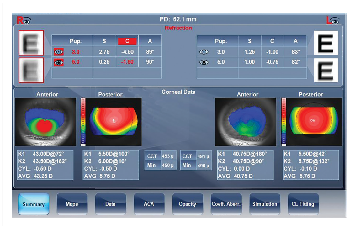
The VX130 summary page shows an overview of findings, note differences in mesopic and scotopic refraction OD, inferior steeping anterior on anterior curvature maps despite normal sim k's OU, and abnormal corneal pachymetry. More in-depth data can be accessed via the VX130 software.
