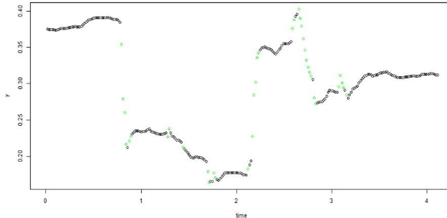
Eye movement on y axis for a sample trial: Dots are highlighted in green if their velocity exceeds 80th percentile. If  $\text{abs}(\tan(Vy/Vx)) > \tan(60) \rightarrow$  Vertical Movement; If  $\text{abs}(\tan(Vy/Vx)) < \tan(30) \rightarrow$  Horizontal Movement (velocity-based threshold algorithm: Salvucci & Goldberg, 2000)
