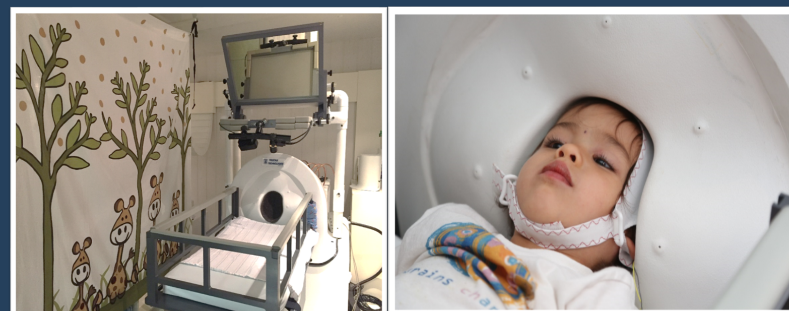
Figure 2. Customized infant MEG system (123-channels gradiometers).
