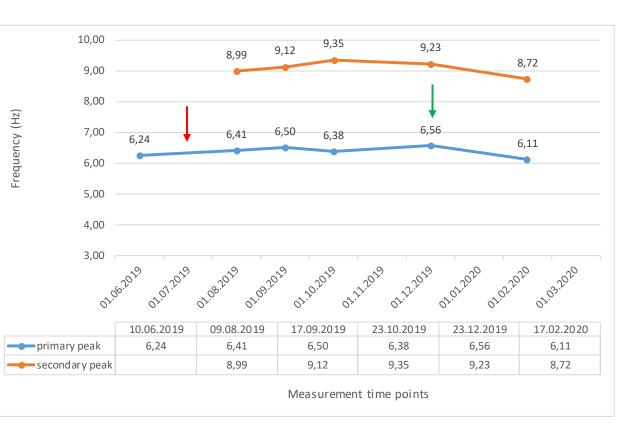
Primary peak – the peak with the highest amplitude in the 3-14 Hz range
