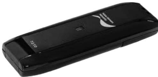
Figure 1.6 Example of a 100 Mbps USB modem – Nokia Siemens Networks 7210.
