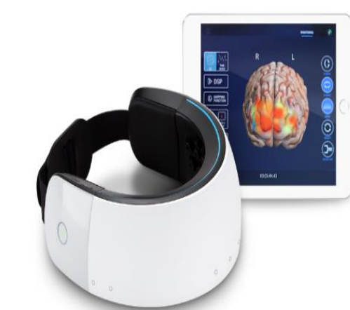
Figure 2. Multi-distance based portable fNIRS device : NIRSIT
