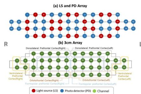
Figure 2. Multi-distance based portable fNIRS device : NIRSIT
